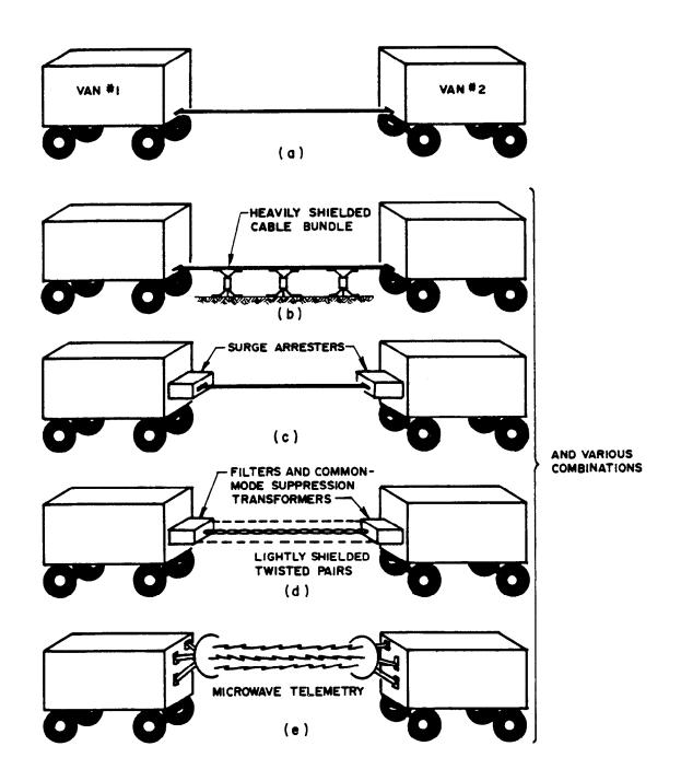
Figure 7-1. Effect of hardening approach on subsystem design.
