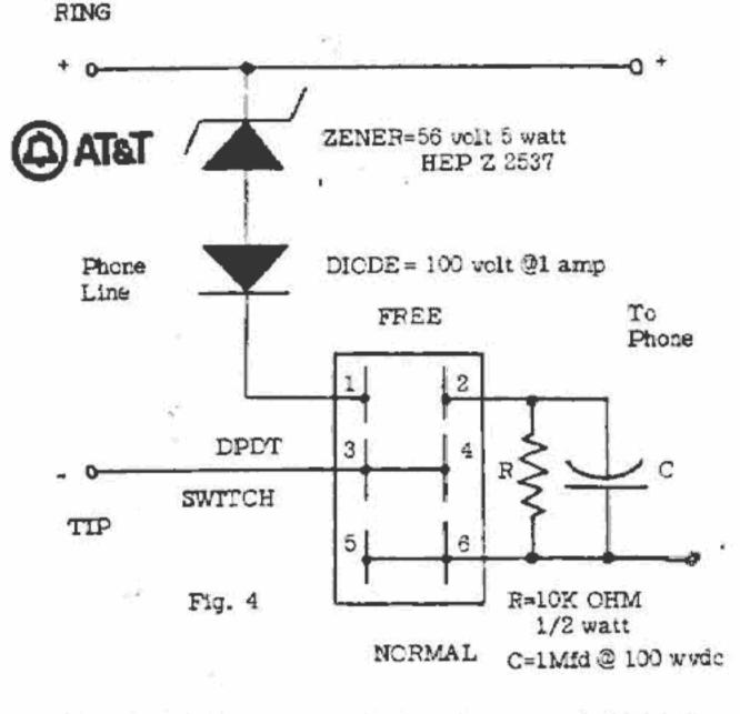
Terminals 3&4 are connected together as are 5&6 but there is no connection between terminals 1&2. With the DPDT switch in the normal position the ringing voltage is across the phone ringer and not across the "answering" diodes. On'y when the switch is put in the "free" position are the diodes placed across the line to momentarily "answer" the phone for a few milliseconds. I cannot think of a more appropriate time to build this improved automatic Black Box:
