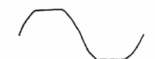
This is a sine wave with its peaks flattened (or cut off). It causes distortion, harshness, and trouble. A telephone earpiece has a dual diode connected across the terminals in newer units, and if the signal level is too great the diodes absorb the peaks of the sine wave, thus causing the waveform to distort like this. Remove the diode before using.
